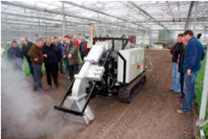
Demonstration of a prototype Agritron, disinfecting greenhouse soil. Source: Koppert Machines.
