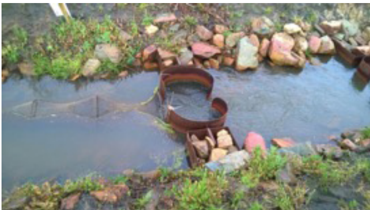
Flow-form with fish trap during the fish feasibility tests. The water flows to the right. The fish swim against the waterflow, so towards the left, they 'jump' through the stairs. Source: Vortex Vitalis.
